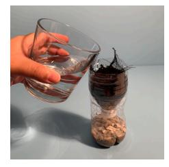
Carefully lift your water table model off the aquifer model and twist off the bottle cap just enough so that it is loose but won't fall off. Set it back on top of the aquifer model and begin to saturate your water table.
